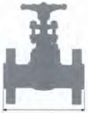
Valve face to face dimension ASME B16.10
